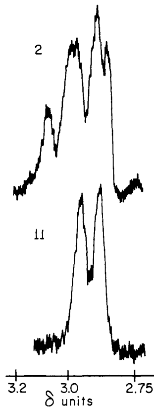
Figure 1. Proton nmr spectra (in CCl_4 ) of H_a region of isotopically normal ( 2 ) and of tetra-deuterated tricyclic amino ketone ( 11 ) ( \delta units from TMS).
